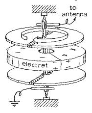
Figure 4. Electrostatic Motor Model
