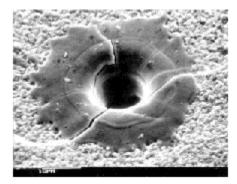
Figure 7. Charge cluster borehole into lead glass. Hole is about 10 micron diameter. Penetration is about 1mm per kV. The slowest speed clocked has been 1 cm in 50 nanoseconds. With an estimated 100 billion electrons carrying 100,000 positive ions, the kinetic energy exceeds 180 microjoules. It has been suggested that a Casmir effect pushes them together, overcoming Coulomb repulsion of like charges. (photo credit: Ken Shoulders)
