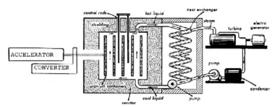
Figure 3. Accelerator Driven Reactor
